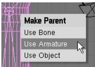
Your next step is to create a **child-parent** relationship between the mesh and the armature with the mesh being the **child** and the armature being the **parent**. Hold down the **shift** key and select the mesh first, then the armature. Press **Ctrl** and **P** to make parent. Select the option to **Use Armature** since the armature is both of the bones together. You will then get some options as to how to create the vertex groups that will move with each bone. Use the **Create**
