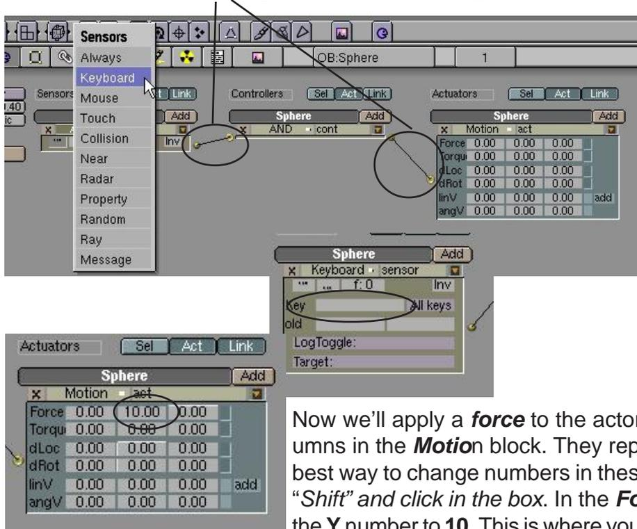
a block for **Key**. click in that box and type the key you want to use. For our case, we’ll use the “**Up Arrow**”. We will tie a force to the up arrow so that when we press it, the sphere will move forward.
