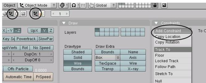
Now, select the **Camera**, go to the **Object** buttons and under **Constraints**, hold down the mouse button on **Add Constraint** and select “Track To”. In the **Track To** options panel, you will see a place for the **Target OB:**. Type in **Actor** here. You will see a dashed line form between the camera and the plane showing the constraint between
