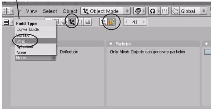
setting to about **20.00**. After you do this, the empty will have some circles displayed on it to represent the wind flow. You may need to rotate the empty so the wind blows toward the particles. As you rotate the empty, you may or may not immediately see the effect of the wind on the particles. Again, you may need to hit the **RecalcAll** button for the sphere.
