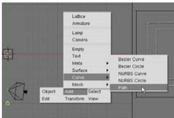
Your first step is to create a **path**. Any type of **Curve** in the **Add** menu can be used as a path, but let's use the **Path** option. Hit the **Space Bar**, select **Add, Curve**, then **Path**. You will then get a path on the screen in **Edit mode** with several points. Shape the path as desired, add more vertices through **Subdivide** if
