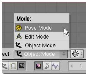
It’s time to animate our “arm” model. To do this we must get into **“Pose Mode”**. Change the Mode option from **Object Mode to Pose Mode**. This can also be done by pressing **“Ctrl”** and **“Tab”** together. Select a bone to work with by RMB clicking on it. Type **“R”** to rotate it. If everything went well, the mesh should move with the bone. Place animation keys in the various frames as before to create an animation.
