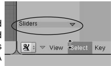
Now, go into **Edit Mode** (**"Tab"** key) and modify the vertices however you want. When you exit edit mode, the slider will now deform the mesh. **To create another slider, insert another mesh key while NOT in edit mode**, then hit **"Tab"** to enter edit mode and modify the mesh. When you again exit edit mode, the slider will be set. Here's an example:
