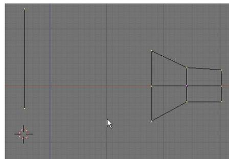
*Bolt and screw threads can be created with a plane shaped into a triangle and the line for spacing set to exactly the same length as the base of the triangle. To make a pointed screw, grab the end thread vertices and scale it with proportional vertex editing ("O") for a nice look.*
