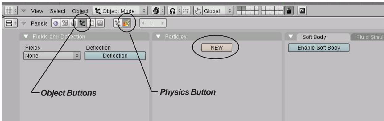
For our example, let's create a **UVSphere** and keep the segments and rings at 32. With the object selected, go to the **Object** buttons, Then select the **Physics Buttons**, click the **"New"** button under the **Particles Panel**. A new particle system will open in the panel and look like this: \_\_\_\_\_
