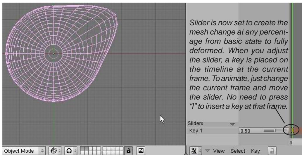
The basic thing to remember about RVKs is that in order to create the slider, **You must insert the key in object selection mode, then enter edit mode (Tab) to modify the mesh.** When you exit edit mode, the slider is set. Repeat the process to create all your sliders.
