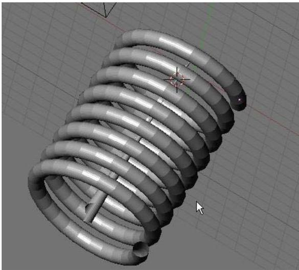
You will notice a shape in the middle of your spring. That shape is created from the vertices you used to designate the length of each loop. You placed this shape in the middle so it is easier for you to select these vertices in edit mode and
