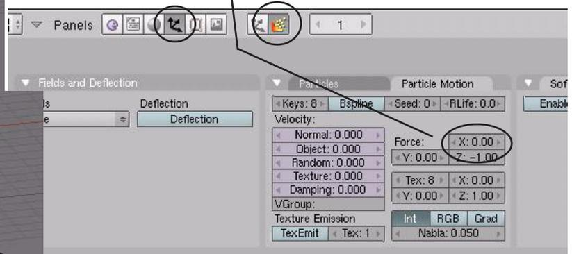
Place your cursor in the 3D window and press “**Alt**”-“**A**” to see the animation. You should see particles drop from the sphere and fall through the plane.
