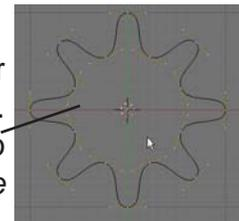
Bezier shapes form differently and use spline points. Experiment with them to get the feel of working with them. Go to the *Edit* buttons and name both objects in the **OB:** block. Finally, select the **Bezier Curve** and go to the *Edit* buttons. You will see a **BevOb:** box. Type the name of the circle there. You will see the shape extruded along the curve!
