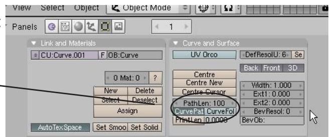
After you press the **Path Follow** button, the camera needs to be rotated and adjusted to the correct direction. After that, it will follow the path.
