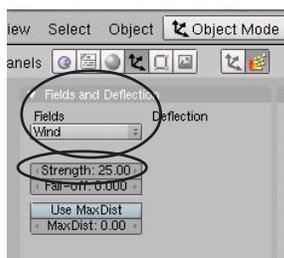
**Empty** to act as the wind. Remember that an empty will not render as an object and works great for this type of application. With the **Empty** selected, go to the **Fields and Deflection** panel and change the Fields to “**Wind**”. Set the **Strength** to about **25**.
