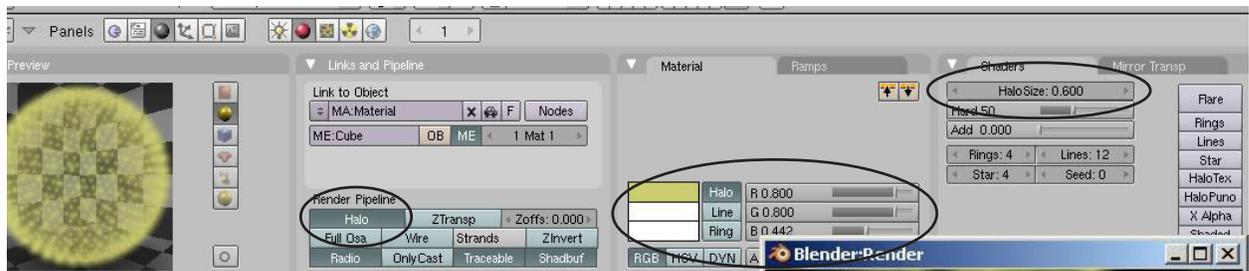
The **halo size** needs to be adjusted for the size of your scene and what you are using the particles to simulate. For example, smoke needs a smaller particle count and a larger **halo setting** and a **Z Transparent and Alpha** setting very low so the smoke looks transparent. Fire may need a higher particle count and a smaller halo setting to look good. Depending on what you want, you can turn on the rings, stars and lines in the halo settings. For a review of Halo settings, refer to page 34.
