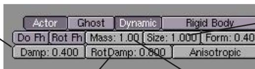
**RotDamp**: rotational dampening- keeps the actor from spinning forever. I like to set this to about 0.8
