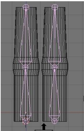
For this example, I've created a mesh we'll call *Finger*. I then created an armature and duplicated both to create 2 fingers. The next step is to **Join** (**"Ctrl" and "J"**) the 2 armatures together, then do the same for both meshes. **Child-parent** the mesh to the armature, select the **"Don't Create Groups"** option.
