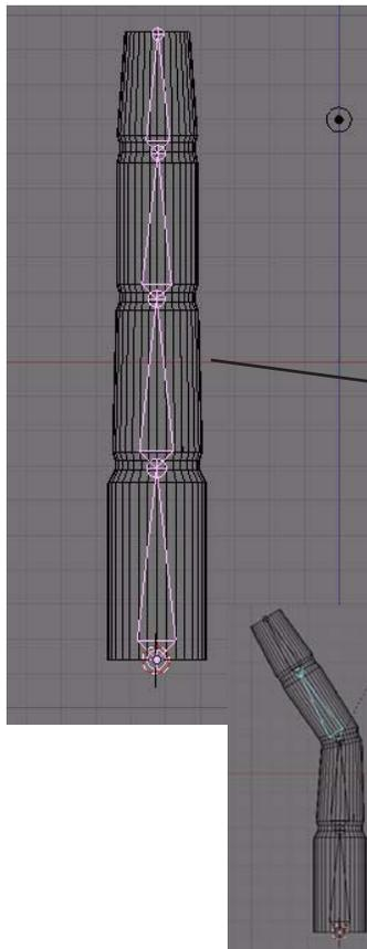
For our example, make a **Cylinder** in the top view, switch to the front view and **Extrude and Scale** the object several times to look like the example.
