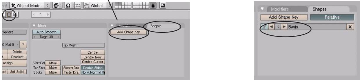
Now press the “**Add Shape Key**” again. The first RVK Slider will be displayed. At this point, enter **edit** mode and modify the mesh. When finished moving vertices, **exit edit mode** (*the vertices will return to their original positions*) and the slider will now be operational. They will also be displayed in the **Action Editor** window.
