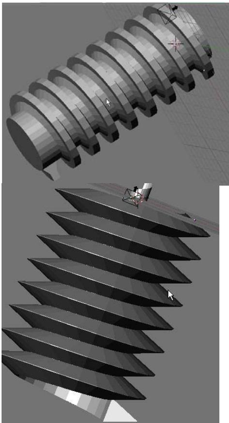
*A Worm Gear created using a subdivided plane as the profile and the line set to equal twice the height of the gear profile. A cylinder has been added through the center to give it a solid appearance.*
